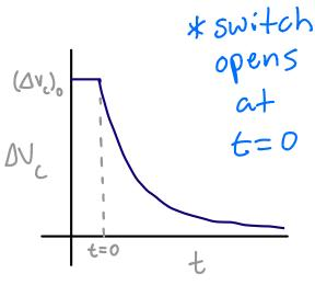
Current and voltage in a discharging RC circuit are mathematically modeled as:
