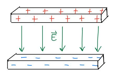
If we connected the two plates in the conductor above, we would see electrons flood towards the positively charged plate. We would also create an electric field within the connecting piece moving from positive to regative:
