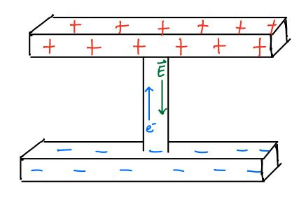
The electric field in the connecting piece creates, and drives, the current. The current can be thought of as the flow of positive charge from the positive plate (terminal) to the negative plate (terminal).
