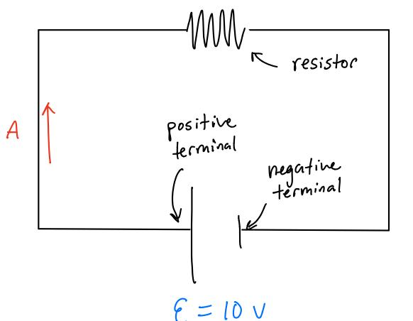
Because E = V = IR, we can substitute IR for e in the previous equation, allowing us to examine how much power the resistor dissipates:
